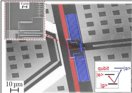
Fig. 1: **Two inductively coupled transmon qubits** leading to a V-shaped energy diagram<sup>1</sup>. Such a system leads to new quantum functionalities such as coherent conversion in time domain and ultrafast high-fidelity qubit read-out.
