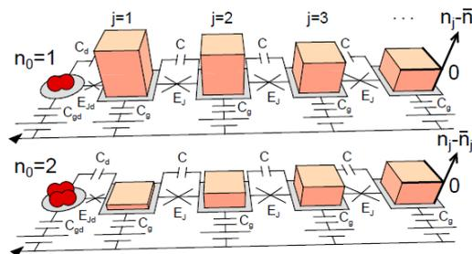
Fig. 4: **Engineering analog quantum simulators** of complex condensed-matter problems, here the widely-sought Kondo screening cloud<sup>5</sup>, in a controlled and tunable experimental setting based on superconducting qubits.
