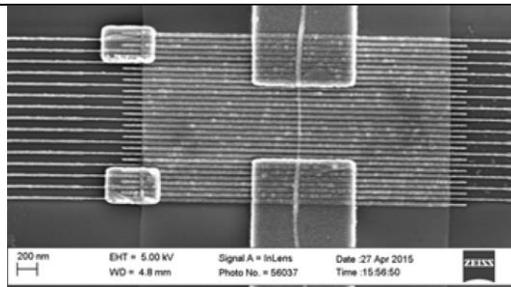
Fig. 3: **Connected SiGe nanowire** sitting on top a series of underneath metallic gates. The two large contact can be superconducting to reveal (quasi) ballistic Andreev levels.<sup>3</sup> A complementary approach is based on electromigrated nano-gaps grafted with a nano-particle.<sup>4</sup>
