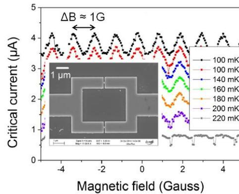
Fig. 2: **Silicon SQUID** showing flux modulation<sup>2</sup>. The superconducting silicon is obtained by using pulse laser annealing for heavily doping bare silicon with boron atoms.
