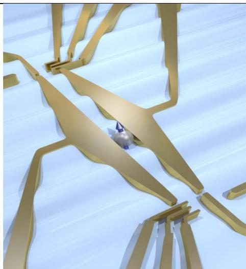
Fig. 3: **On-demand displacement of a single electron spin.** A single electron spin, trapped initially in the left quantum dot, is propelled by a sound wave towards the second quantum dot, at a distance of 4 microns.<sup>3,4</sup>
