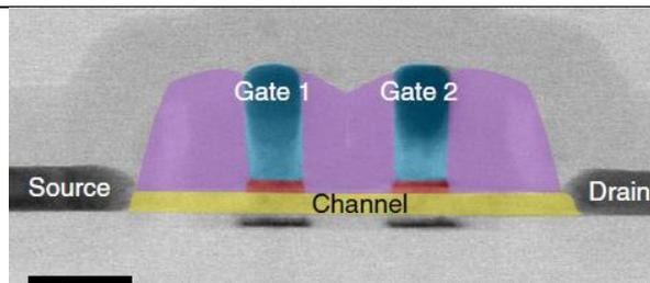
Fig. 2: **A spin qubit in a CMOS-Si-transistor** where individual electrons are trapped underneath each gate.<sup>2</sup> (scale bar=50 nm)
