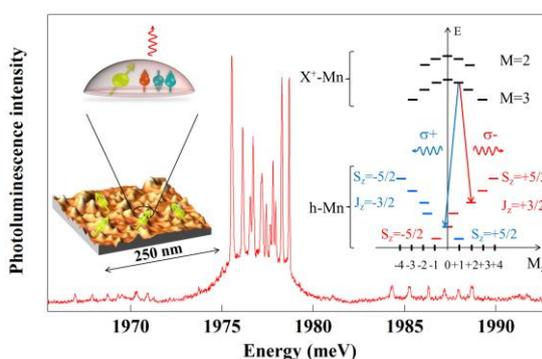
Fig. 4: **Optical control of an individual Mn atom in a semiconductor quantum dot.** The optical absorption and emission of the quantum dot are exploited to initialize and to read out the spin state of the magnetic atom.<sup>5</sup>
