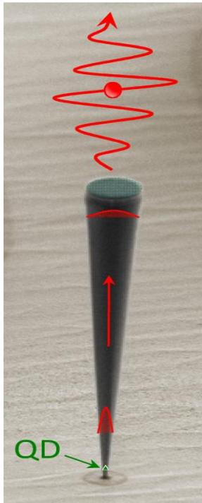
Fig. 1: **Single-photon source:** a semiconductor quantum dot (QD) embedded in a photonic waveguide with tailored ends, offers efficient light emission<sup>1</sup> and giant non-linearities.<sup>2</sup>
