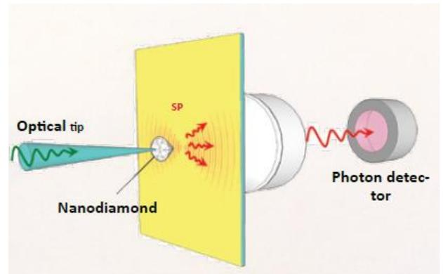
Fig. 4: **Quantum plasmonics:** a single NV center in a diamond nanocrystal at the tip of a near-field scanning optical microscope creates individual surface plasmons (SP) in a metal film.<sup>6</sup> Plasmonic nanoantennas can also be tuned to enhance the linear and nonlinear processes at the nanoscale.<sup>7</sup>
