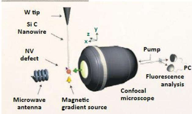
Fig. 3: **Hybrid mechanical systems:** a mechanical oscillator is coupled to an individual quantum system, such as an NV center in diamond<sup>4</sup> or a quantum dot,<sup>5</sup> for quantum information storage or sensing.
