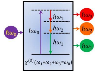
Fig. 2: **Triple photon generation** governed by the third-order susceptibility  $\chi^{(3)}$  in a nonlinear medium<sup>3</sup> and the Wigner function for a three-photon quantum state.
